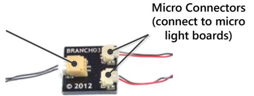
The BRANCH03 adapters in this kit are designed to convert the micro connectors to standard connectors. Make sure to insert the micro plugs into the correct connector on the BRANCH03 adapter board as shown in the photo above.
