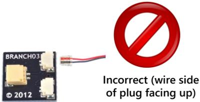
When inserting the micro plugs into the micro connectors, make sure to insert the right way (the plug will only fit one way). Note the appearance of the plug in the photos to the right. **Do not force!**
