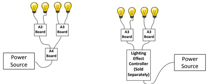
Using a combination of BRANCH03 (A3) boards, BRANCH04 (A4) boards, and the connecting cables, you can connect your lights in many configurations— a 3xAA battery pack (if included with this kit) will power over 100 LEDs. Add a Lighting Effect Controller to make your lights flicker, flash, strobe, or pulse.
